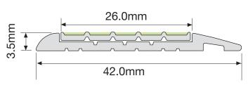
The T2-103 Step Edging is designed to ensure visibility of steps in escape routes for compliance with NFPA 101 Life Safety Code (NFPA) and International Fire Code (IFC), and any performance based building codes. T2-103 can be used on steps in the following ways: (1) to mark the front edge of steps; (2) to mark the sides of steps. The Step Edging will be effective in all light conditions including during failure of the main lighting.
